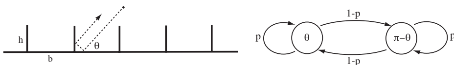
Figure 2. Transition probabilities for this “fence microgeometry” are given by the above Markov diagram. Standard random walk on \mathbb{R} ( p = 1/2 ) corresponds to the projection of the random flight in a channel of radius r = 1/2 , \theta = \pi/4 , and b/h = 4 .
